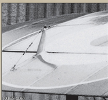
Control horn detail from Sopwith built Snipe E8044
