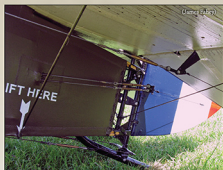
Tailplane and tail skid detail from reproduction Sopwith Snipe E8102.
