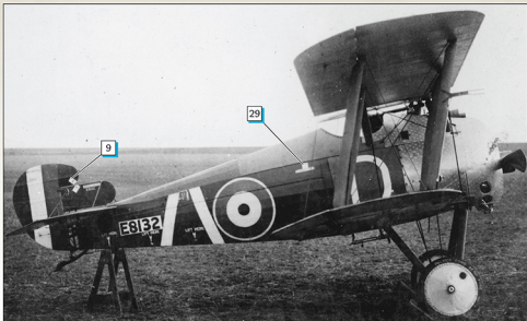
Sopwith built Snipe E8132 "D" of 208 Sqn is from the same production order as Barker's E8102 and conveniently displays much of its numerous stenciling and inspection marks, although it too is missing the Sopwith factory decals commonly applied to the struts and side of the fuselage. The unpainted aluminium cowls and shields have a turned finish unlike Barker's E8102 which have been overpainted in a PC10 equivalent enamel paint. E8132 was delivered to 208 Sqn at Maretz on 3 November and marked with the 'angled bar' squadron markings and individual identification letter D of A flight as shown here and was written off following a crash which injured the pilot, CR Davidson (possibly 6 victory ace Charles Robert Davidson who had previously served with 14 and 111 Sqn).
